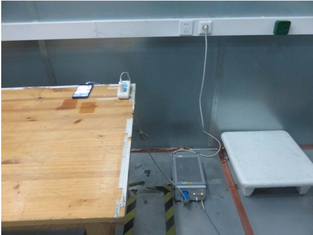
Picture 2 Conducted Emission Test Setup
