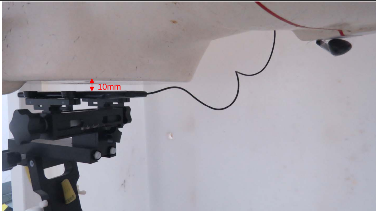
Picture 13: Back Side with Earphone, the distance from handset to the bottom of the Phantom is 10mm
