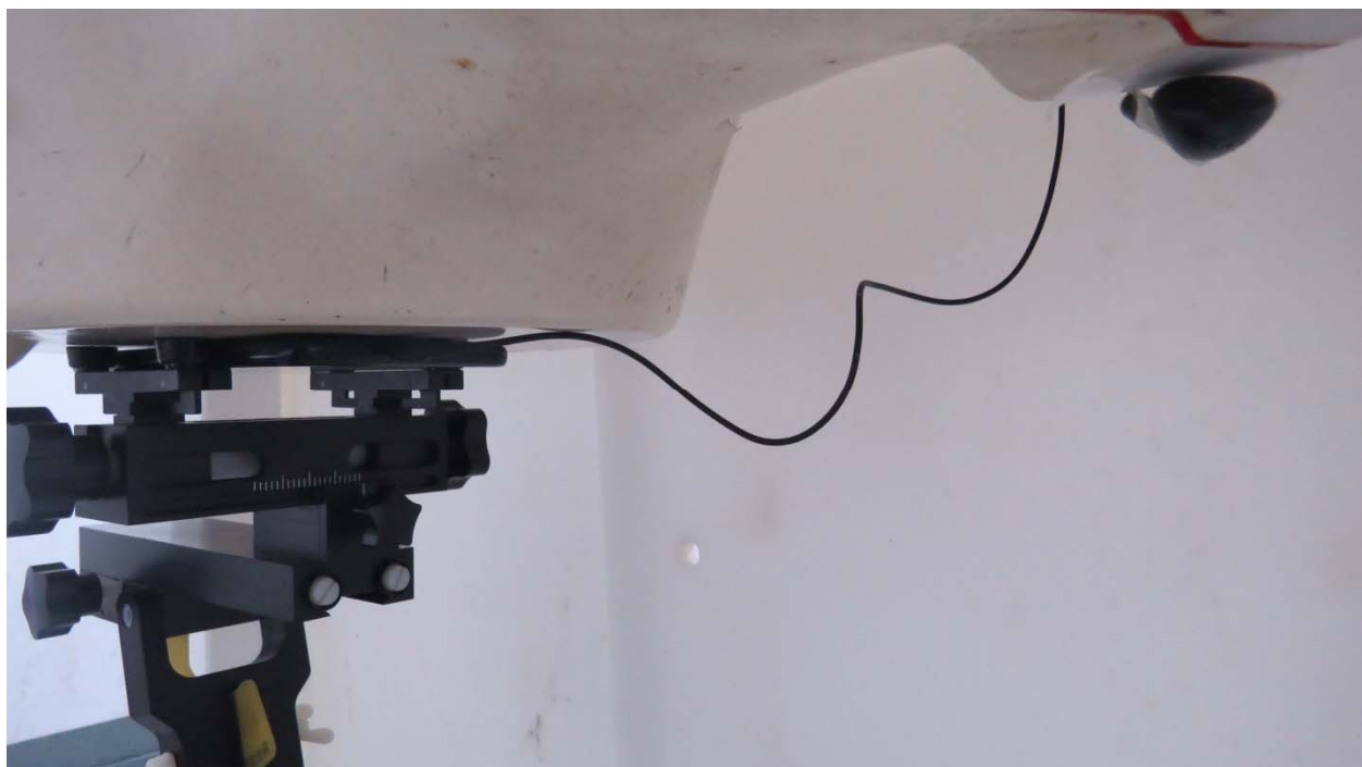
Picture 14: Back Side with Earphone, the distance from handset to the bottom of the Phantom is 0mm
