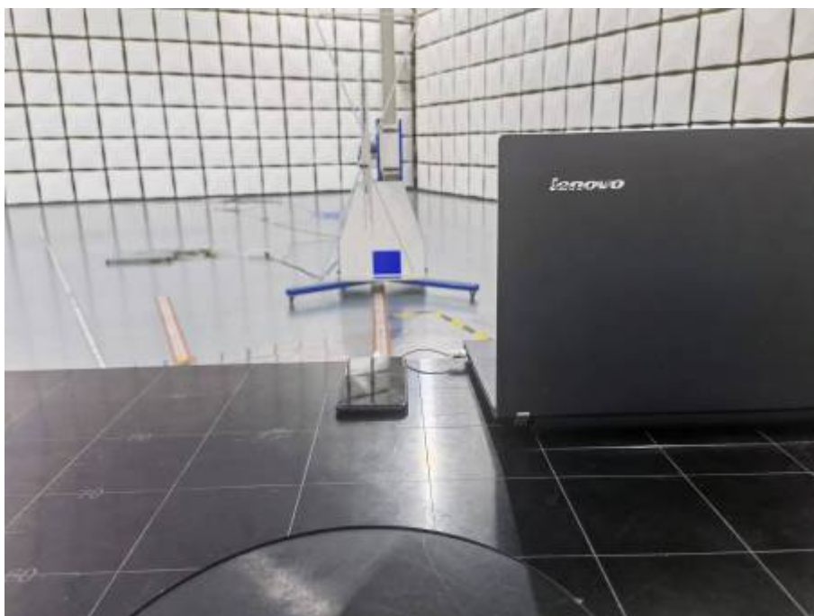
Radiated Emissions Test Setup (with laptop) (30-1000MHz)
