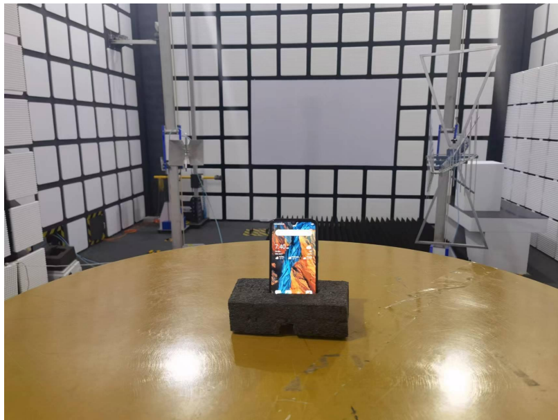
Spurious Radiated Emissions Test setup
