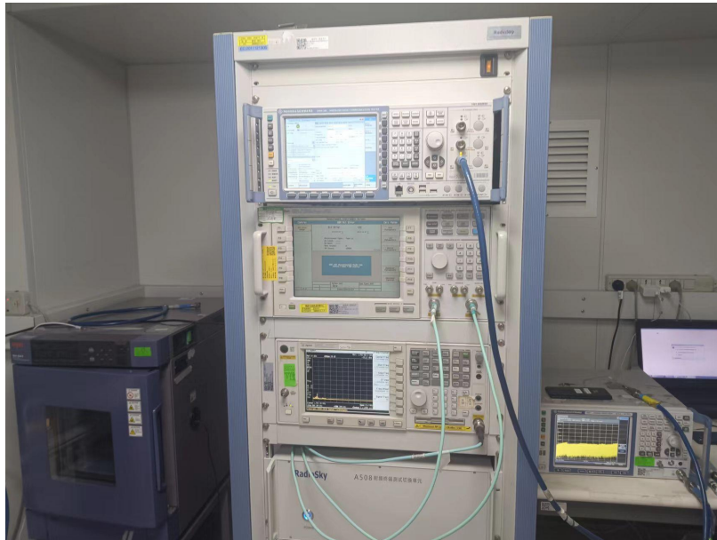
RF Conducted Test setup (GSM/WCDMA/LTE/BT/WIFI)
