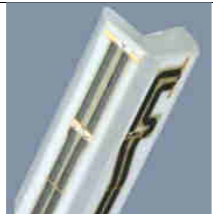
Fig 5.2 Photo of E-field Probe
