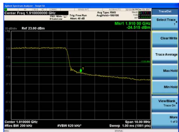
LTE Band 2 5MHz 16QAM 1RB CH-High
