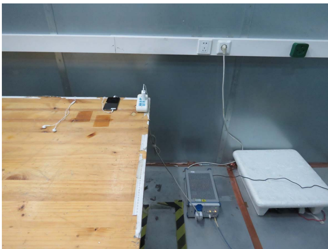
Picture 2 Conducted Emission Test Setup
