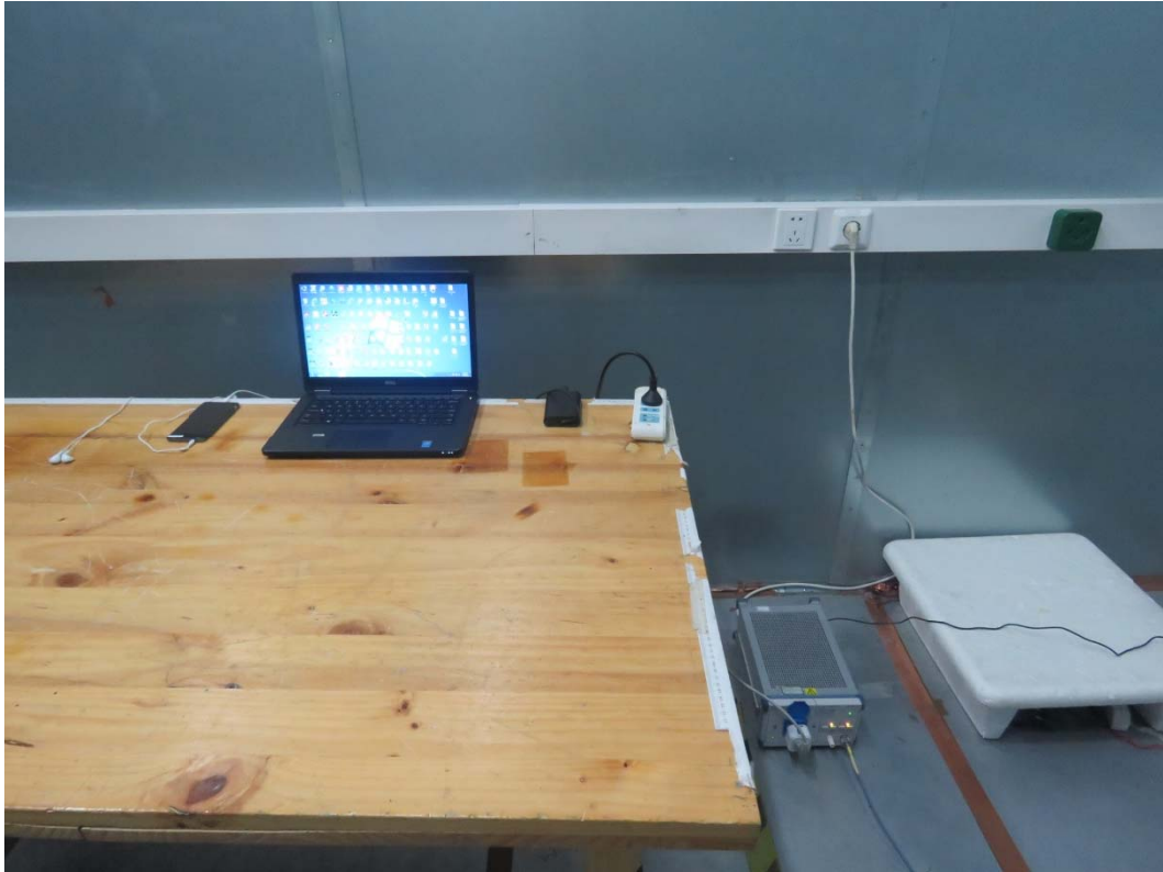
Picture 2 Conducted Emission Test Setup
