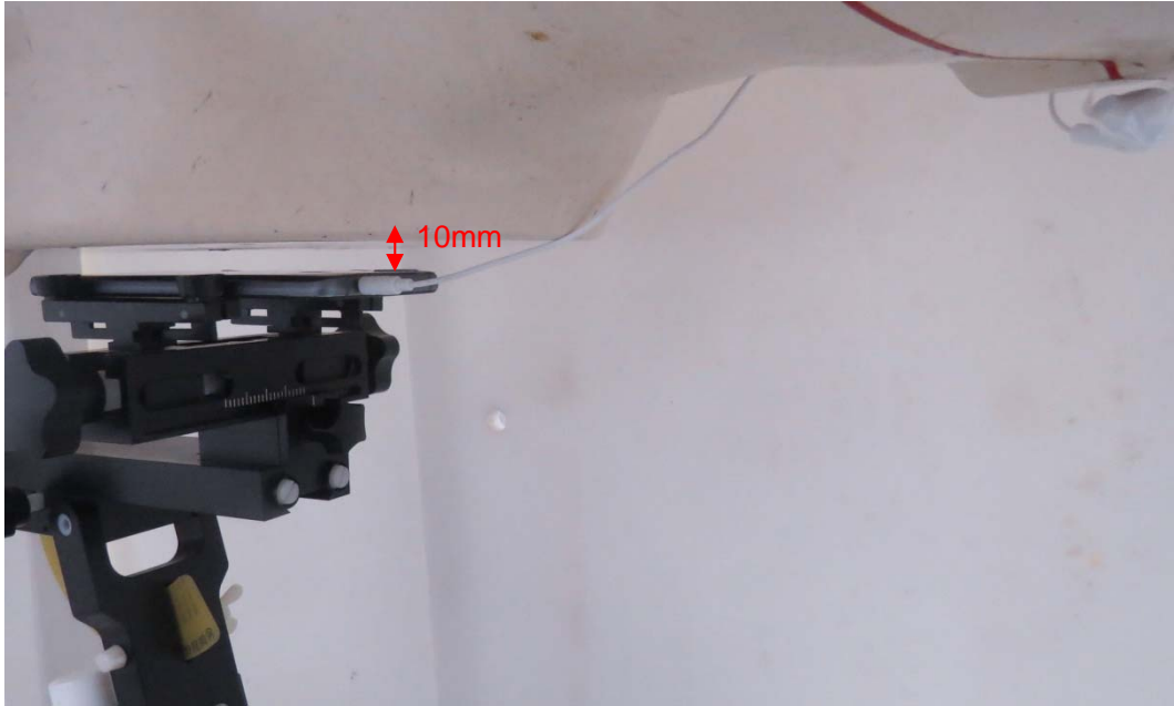
Picture 11: Back Side, the distance from handset to the bottom of the Phantom is 10mm
