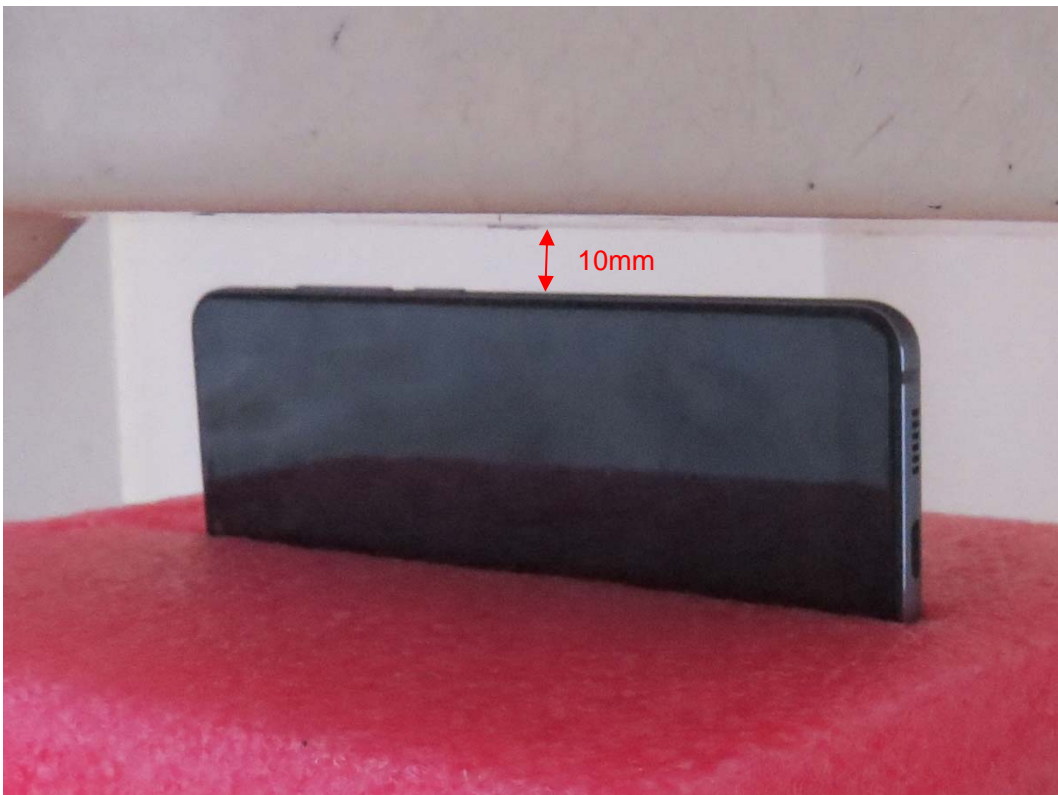
Picture 8: Right Side, the distance from handset to the bottom of the Phantom is 10mm
