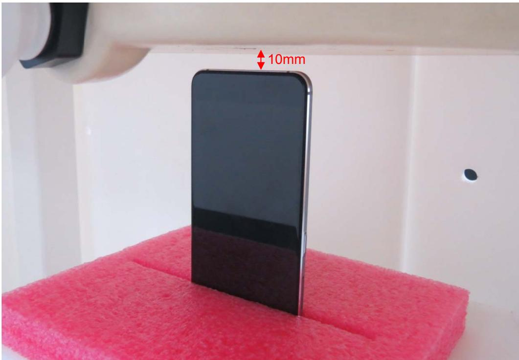
Picture 21: Bottom Edge, the distance from handset to the bottom of the Phantom is 10mm
