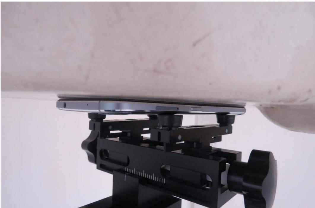
Picture 23: Front Side, the distance from handset to the bottom of the Phantom is 0mm
