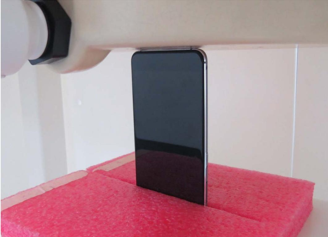
Picture 24: Bottom Edge, the distance from handset to the bottom of the Phantom is 0mm
