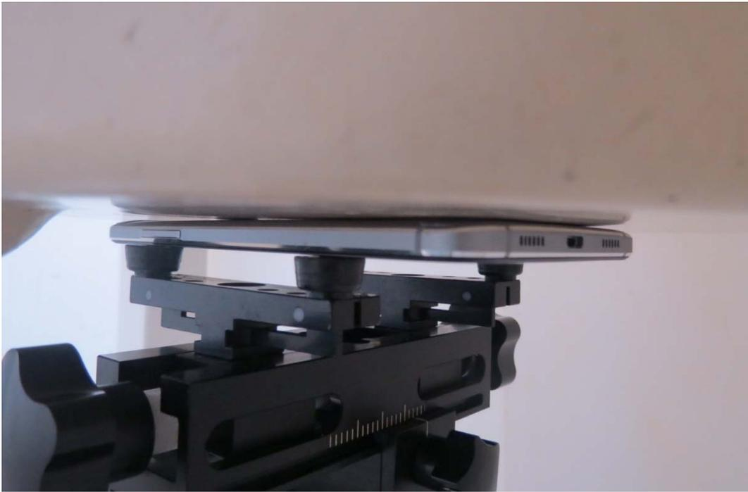
Picture 22: Back Side, the distance from handset to the bottom of the Phantom is 0mm
