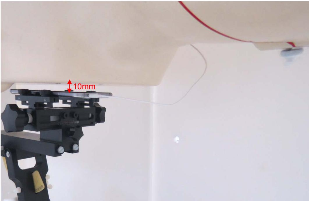
Picture 25: Front Side with Earphone, the distance from handset to the bottom of the Phantom is 10mm
