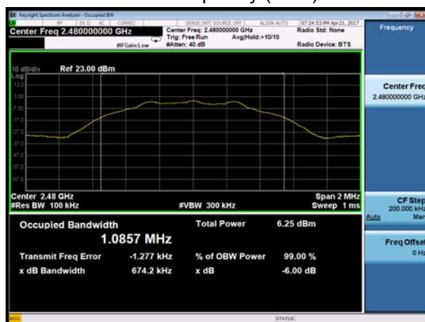
BLE Carrier frequency (MHz): 2480
