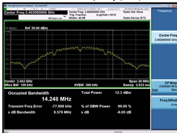
802.11b, Carrier frequency (MHz): 2462
