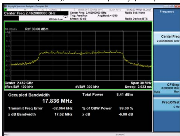
802.11n(HT20), Carrier frequency (MHz):2462
