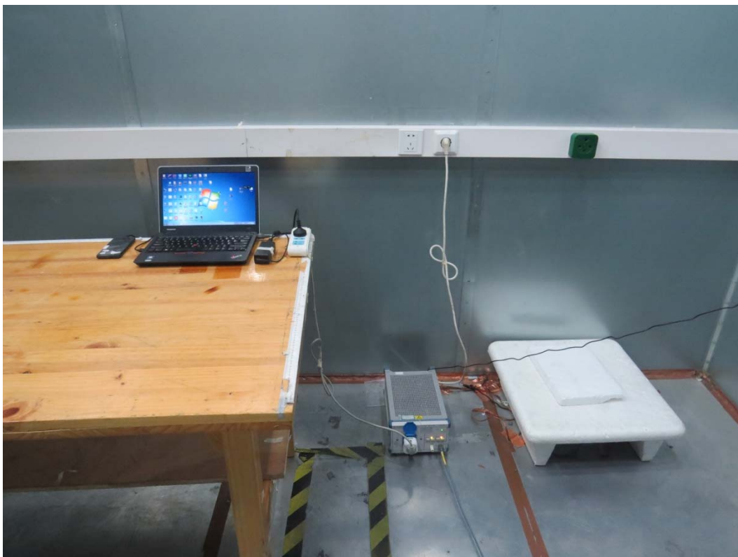
Picture 3 Conducted Emission Test Setup
