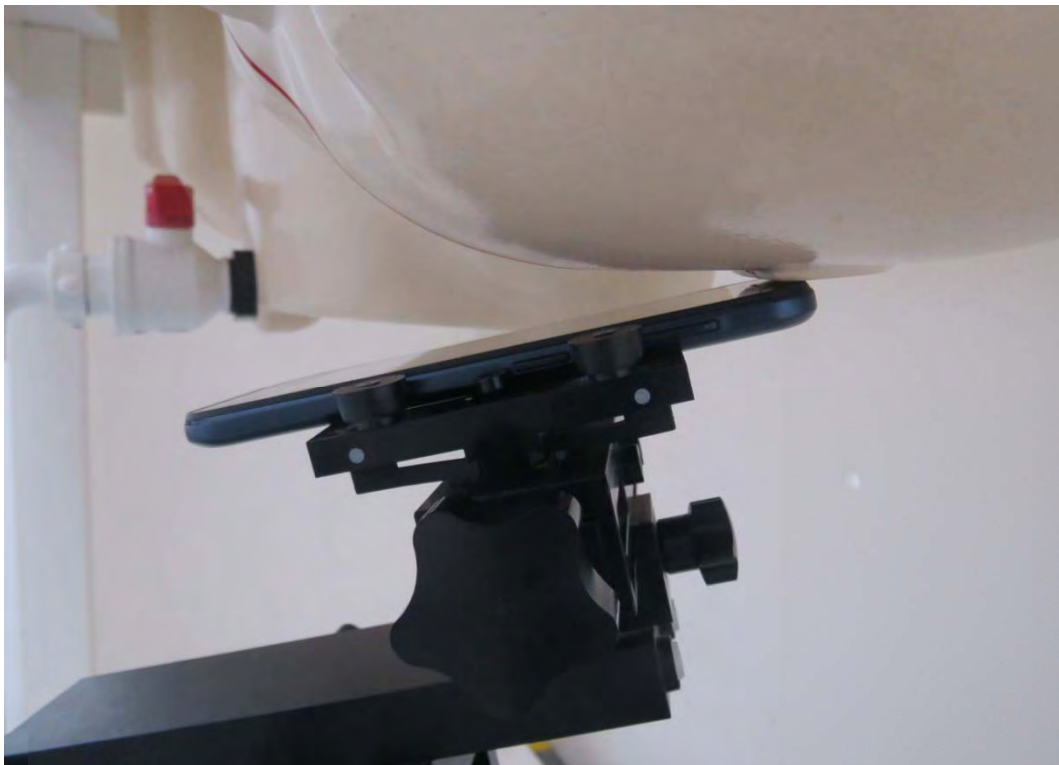
Picture 13: Left Hand Tilt 15 Degree Position
