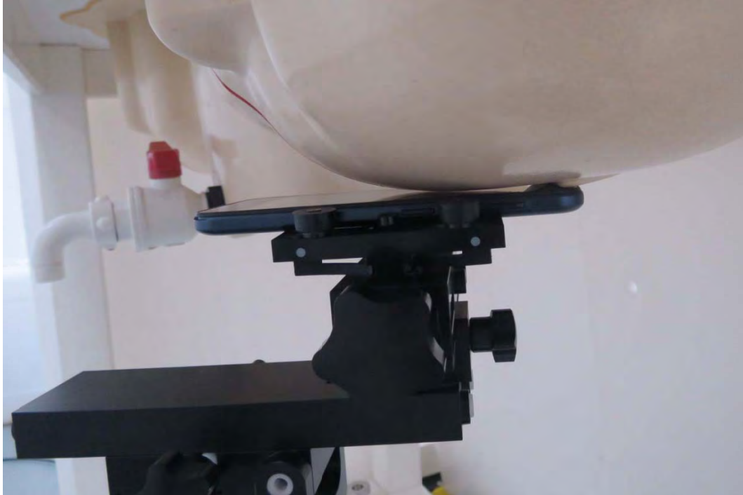
Picture 12: Left Hand Touch Cheek Position
