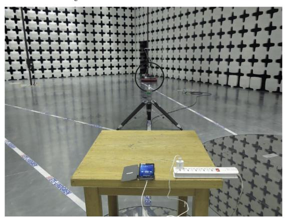
2. Part 15C Field Strength Measurement above 30MHz
