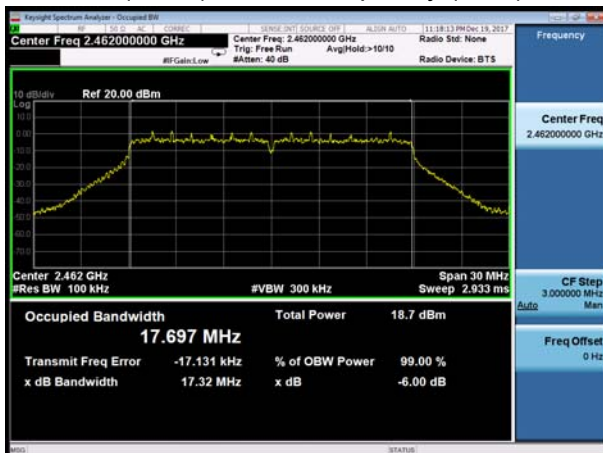
802.11n(HT20), Carrier frequency (MHz): 2462
