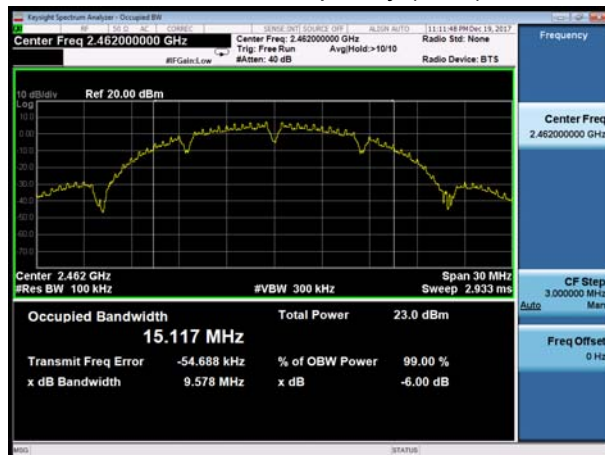
802.11b, Carrier frequency (MHz): 2462
