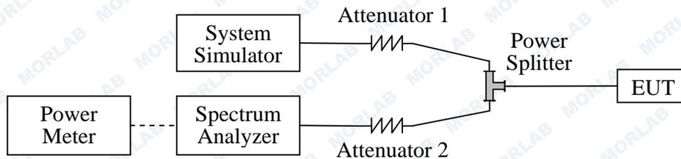
The EUT, which is powered by the Battery, is coupled to the Spectrum Analyzer (SA) and the System Simulator (SS) with Attenuators through the Power Splitter; the RF load attached to the EUT antenna terminal is 50Ohm; the path loss as the factor is calibrated to correct the reading. The EUT is commanded by the SS to operate at the maximum output power i.e. Power Control Level (PCL) = 5 and Power Class = 4. A call is established between the EUT and the SS.
