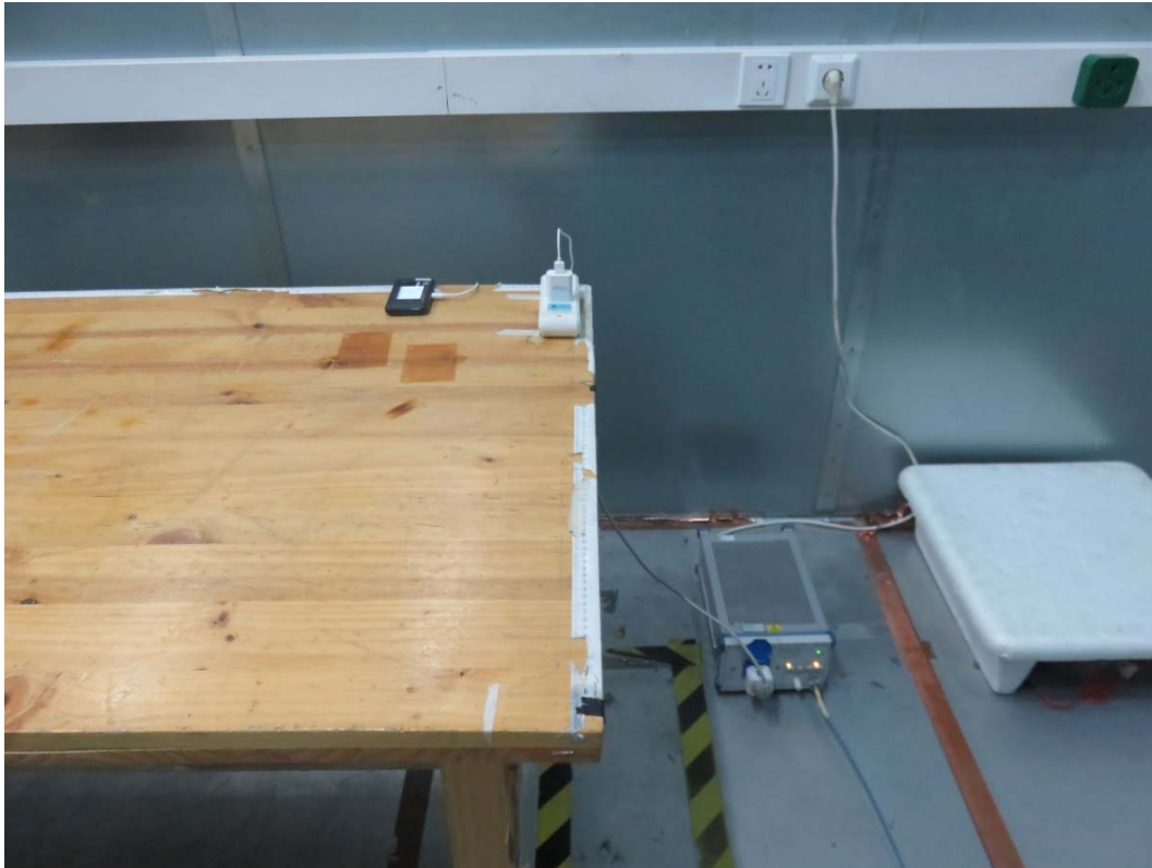
Picture 2 Conducted Emission Test Setup
