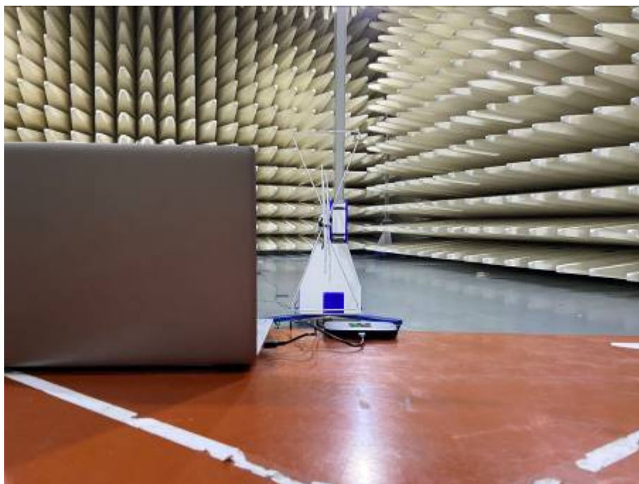
Radiated Emissions Test Setup (with laptop) (30-1000MHz)
