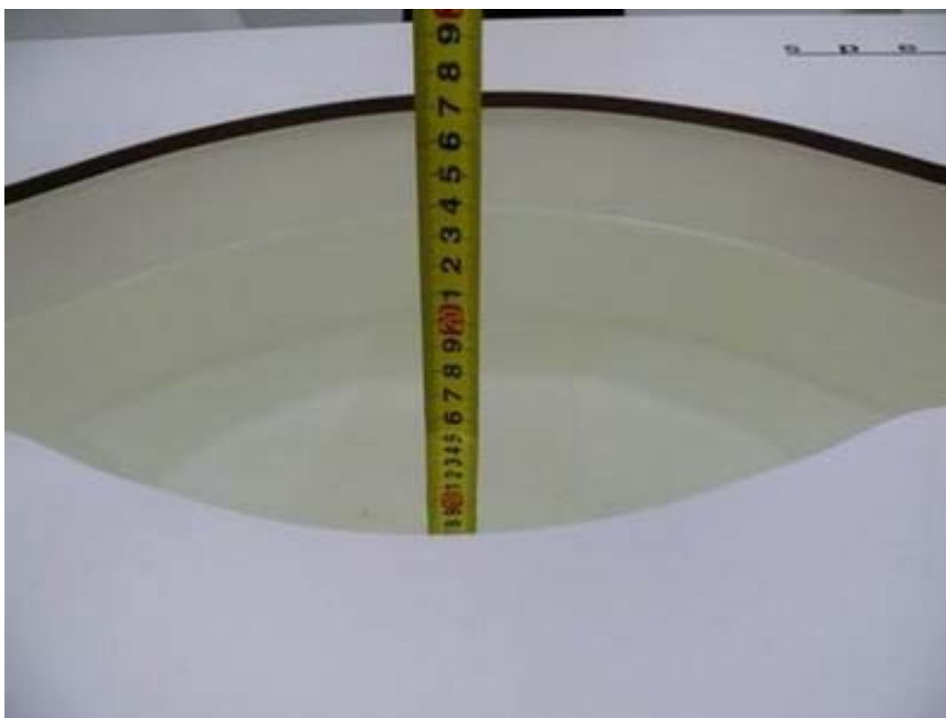
Picture 4: Liquid depth in the flat Phantom (1750 MHz, 15.2cm depth)
