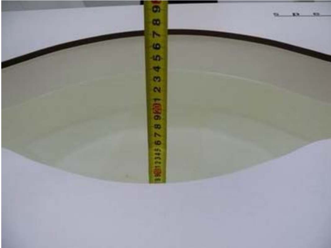
Picture 7: Liquid depth in the flat Phantom (2600 MHz, 15.3cm depth)
