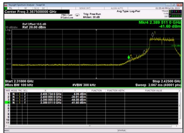
,Plot 2,Band Edge-802.11g,2437MHz ,Ant1
