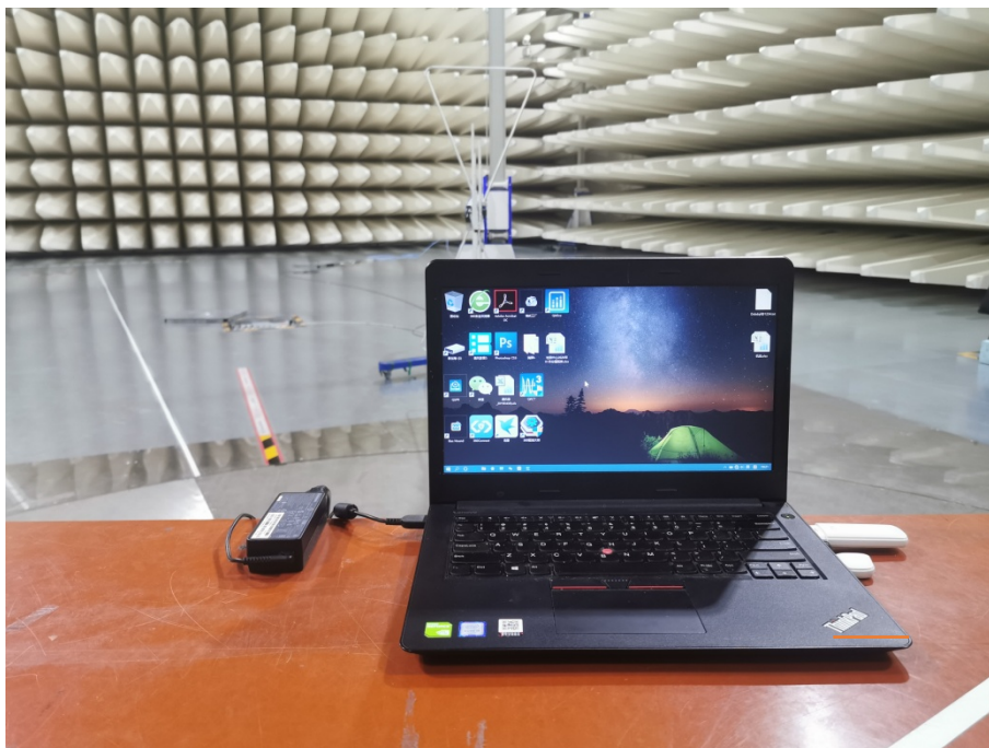
Spurious Radiated Emissions Test setup (below 1GHz)
