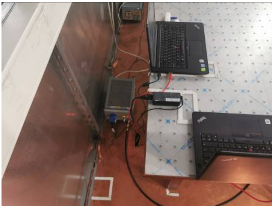
Conducted Emissions Test Setup (with charger)
