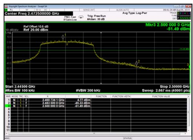
,Plot 2,Band Edge-802.11g,2462MHz ,Ant1
