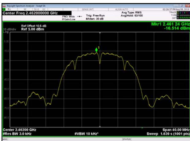
Power spectral density-802.11b ,2462MHz,Ant0
