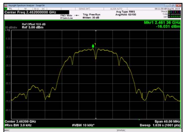
Power spectral density-802.11b ,2462MHz,Ant1
