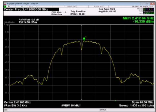
Power spectral density-802.11b ,2437MHz,Ant1
