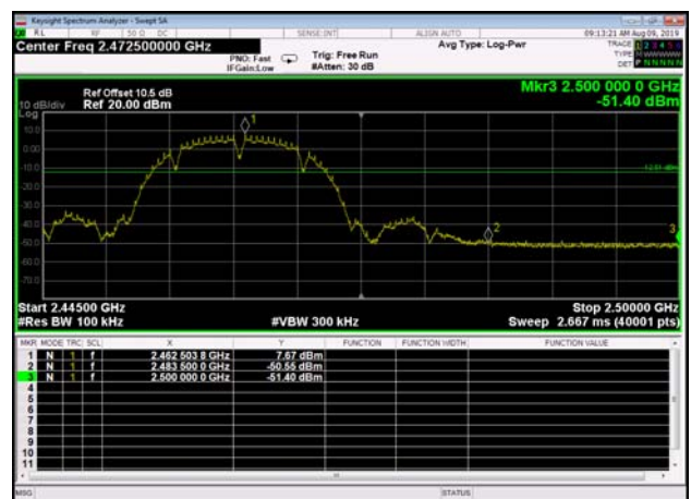
,Plot 2,Band Edge-802.11b,2462MHz ,Ant1
