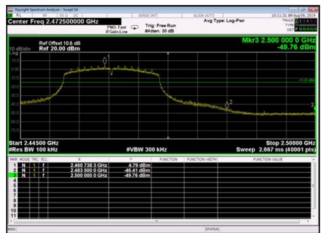
,Plot 2,Band Edge-802.11n(HT20) ,2462MHz,Ant1
