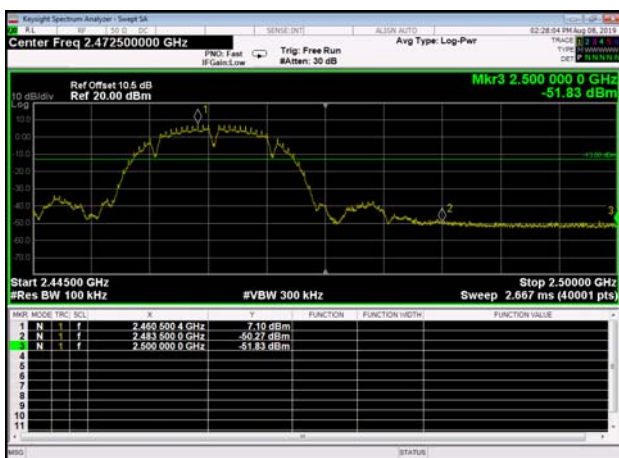
,Plot 2,Band Edge-802.11b,2462MHz ,Ant0
