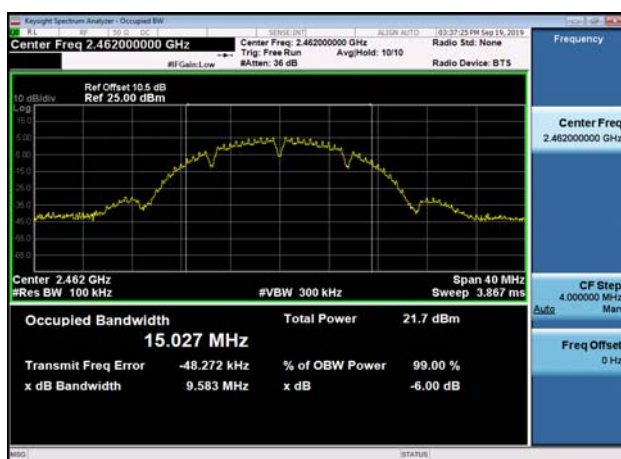
6dB Bandwidth-802.11b,2462MHz,Ant0
