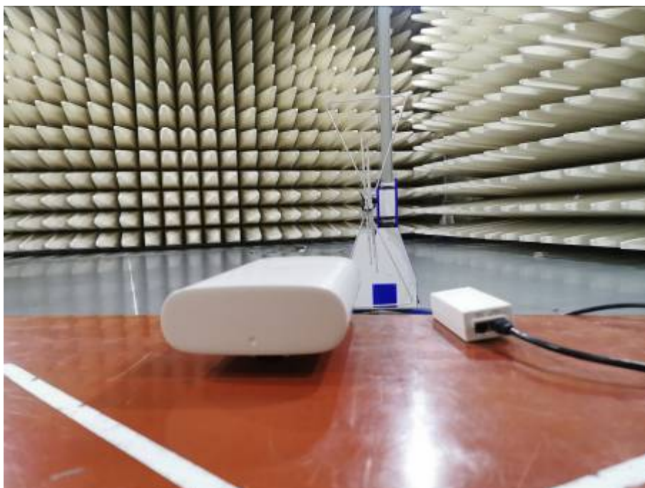
Radiated Emissions Test Setup (30-1000MHz)
