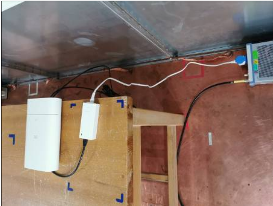
Conducted Emissions Test Setup
