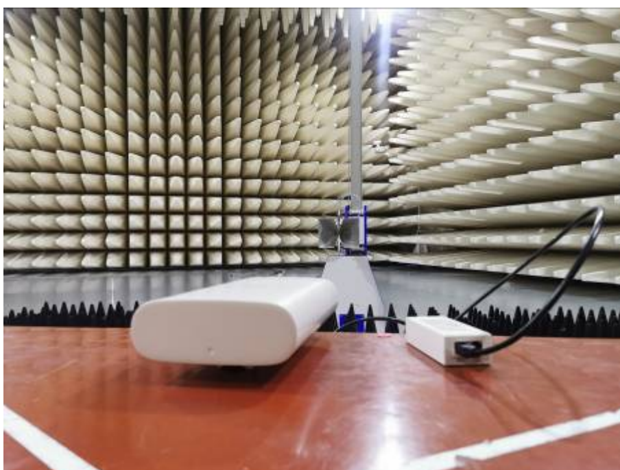
Radiated Emissions Test Setup (above1GHz)
