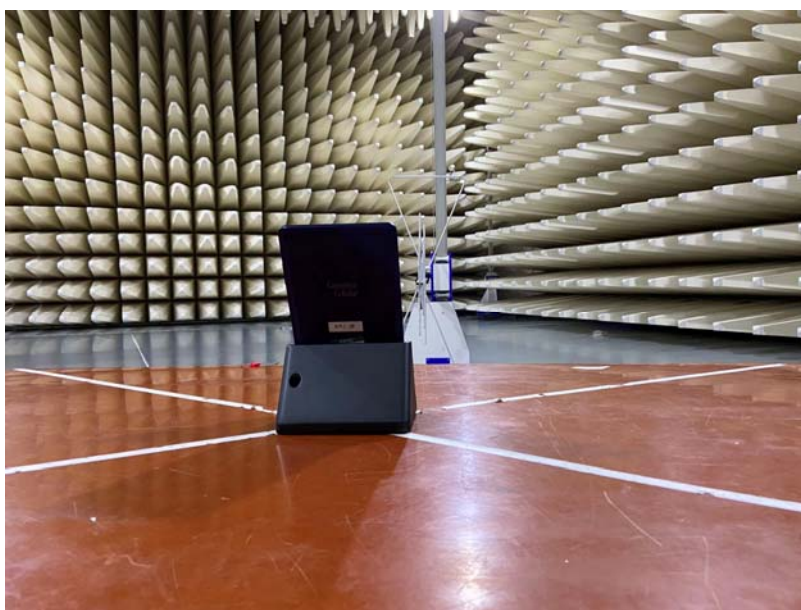
Radiated Emissions Test Setup(below 1GHz)
