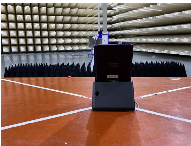
Radiated Emissions Test Setup (above1GHz)
