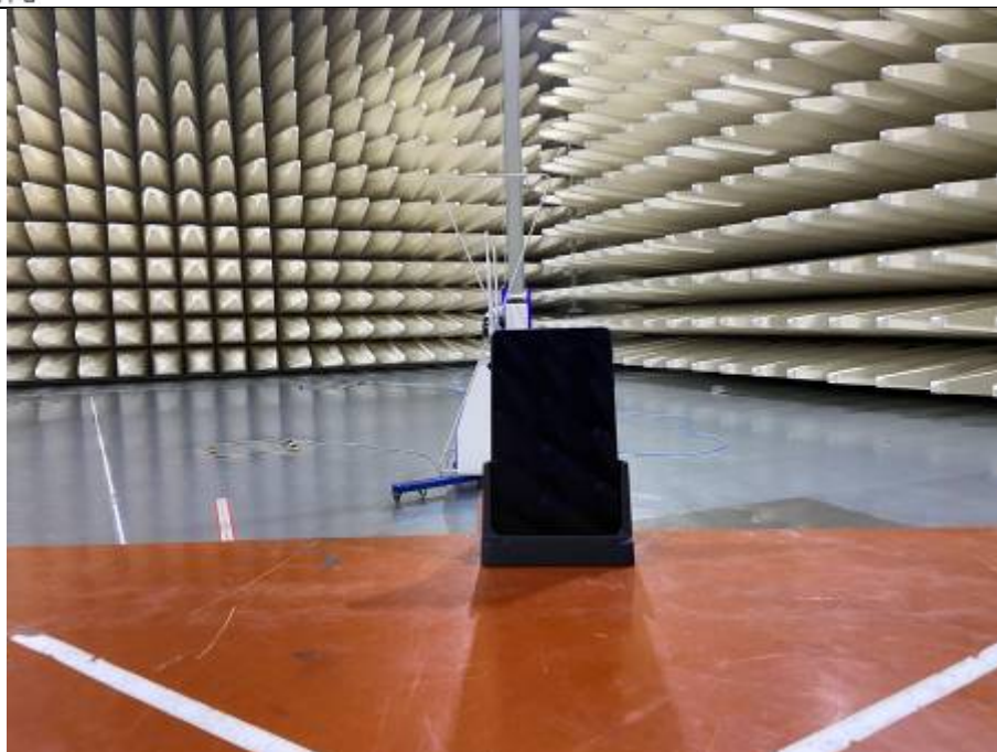
Radiated Emissions Test Setup (with charger) (30-1000MHz)
