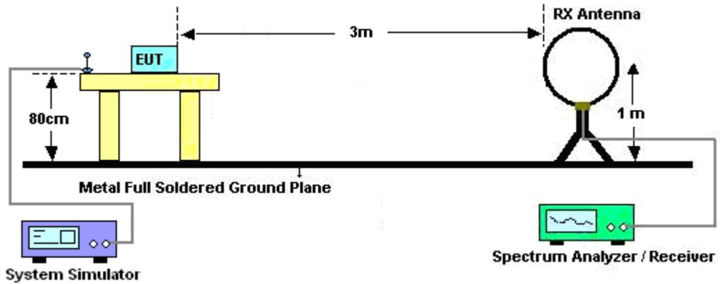
For radiated emissions from 30MHz to 1GHz
