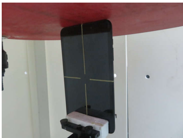
Edge1, Test Separation 0 mm
