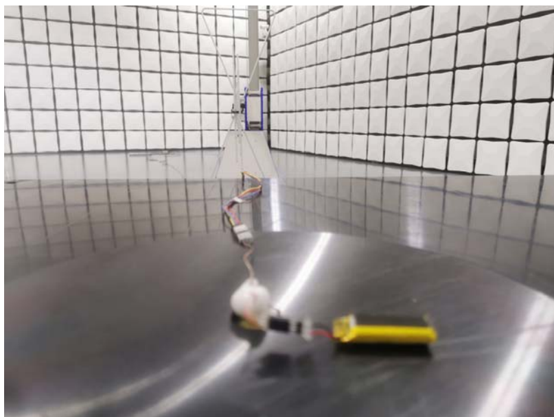
RF Conducted Test setup (BT)
