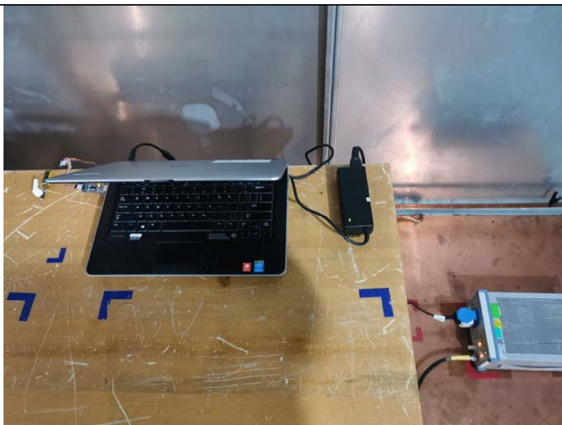
Conducted Emissions Test Setup (with charger)
