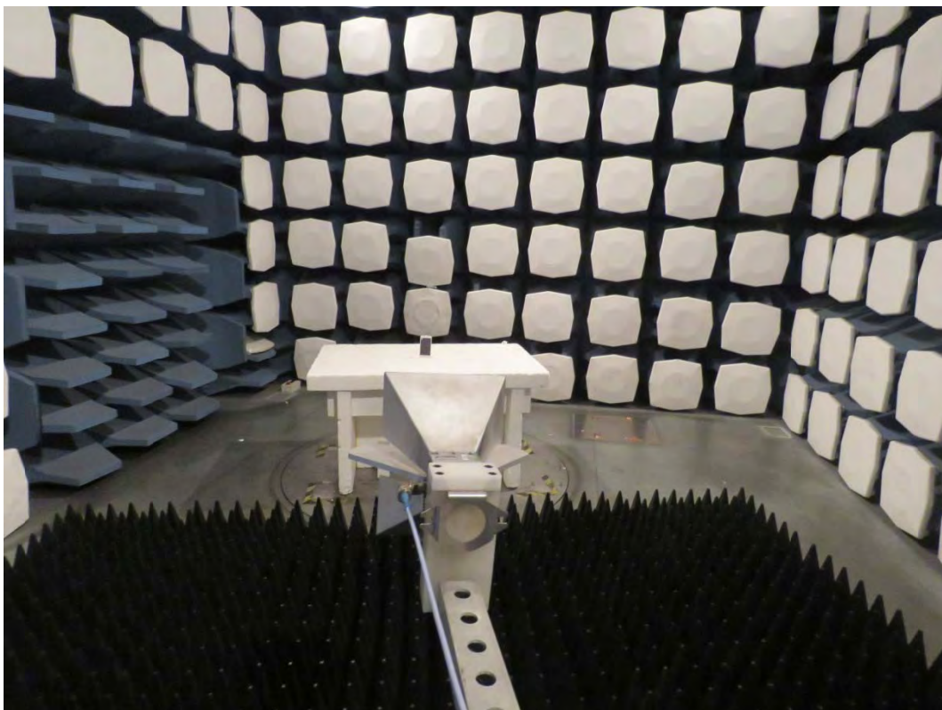
Picture 2: Radiated Spurious Emissions Test setup
