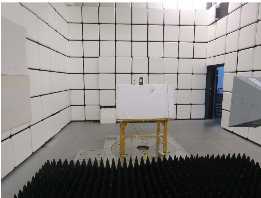
Picture 1: Radiated Spurious Emissions Test setup
