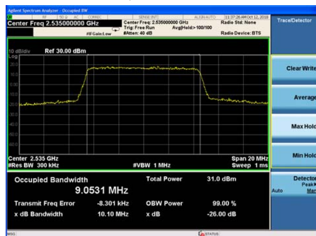
LTE Band 7 QPSK 20MHz CH-Middle
