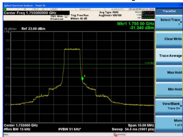
LTE Band 4 QPSK 3MHz CH-High, 1 RB
