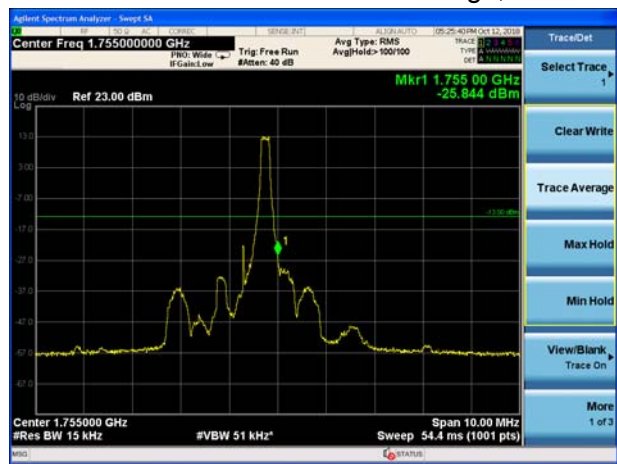
LTE Band 4 QPSK 1.4MHz CH-High, 100%RB
