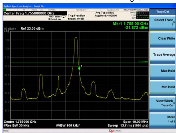
LTE Band 4 QPSK 3MHz CH-High, 1 RB
