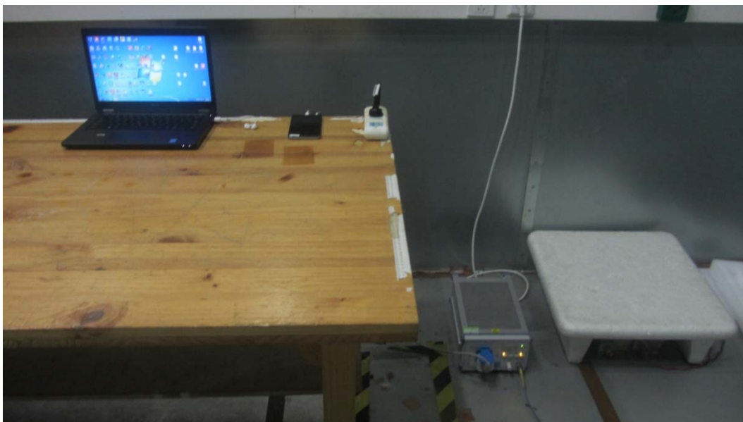
Picture 2 Conducted Emission Test Setup
