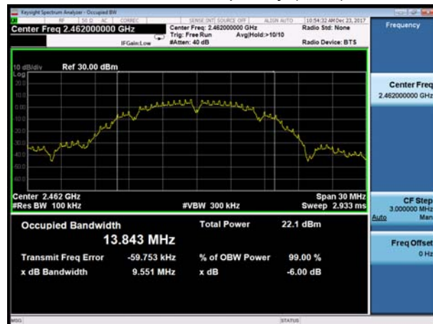
802.11b, Carrier frequency (MHz): 2462
