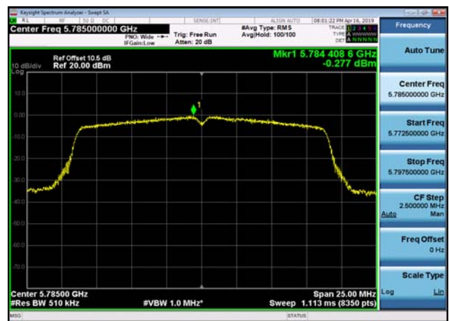
U-NII-3 Power spectral density-802.11 ac(20MHz),5785MHz
