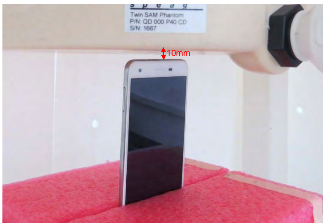
Picture 18: Top Side, the distance from handset to the bottom of the Phantom is 10mm
