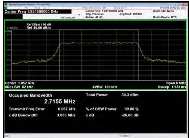
LTE Band 2 1.4MHz 16QAM CH-Middle
