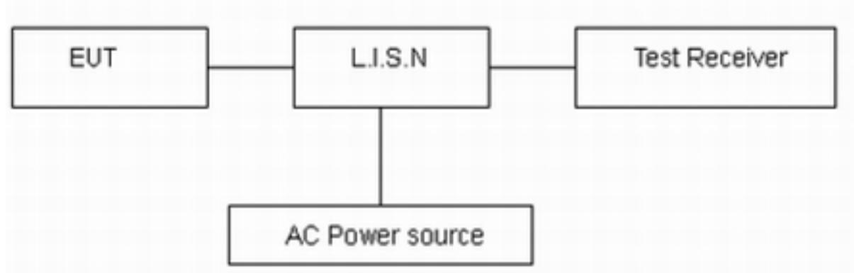
Note: AC Power source is used to change the voltage 110V/60Hz.
