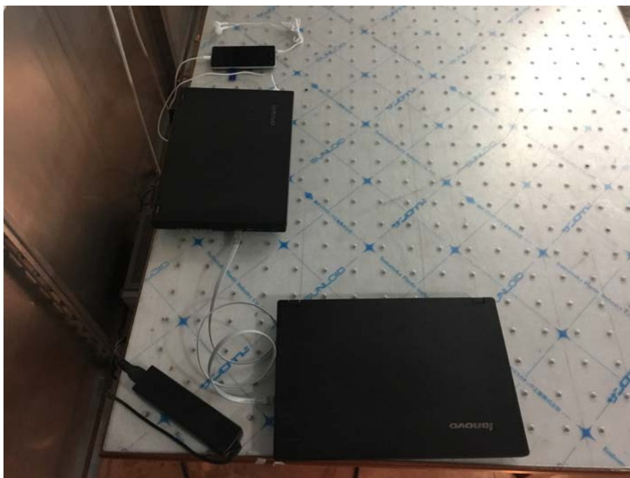
Conducted Emissions Test Setup (with laptop)
