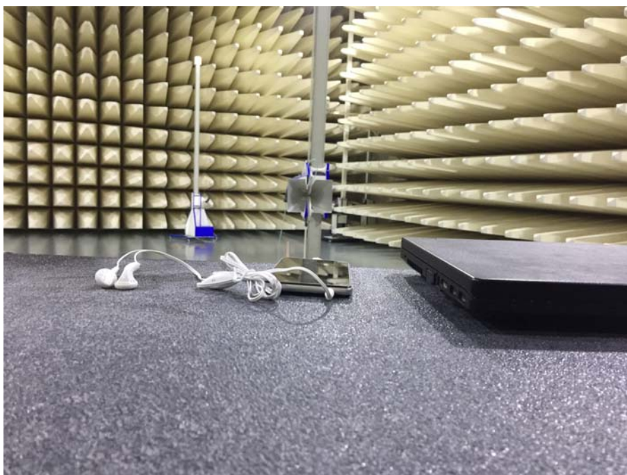
Radiated Emissions Test Setup (with laptop)
