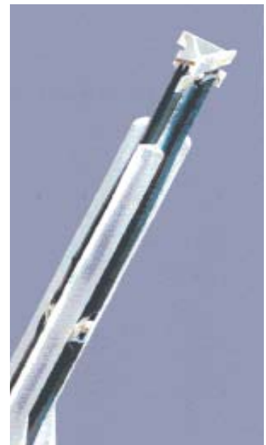
Inside view of ES3DV2 E-field Probe
