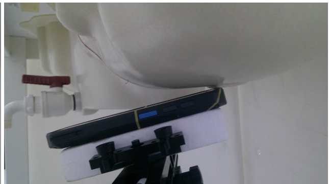
Left Tilted, Test Separation 0 mm
