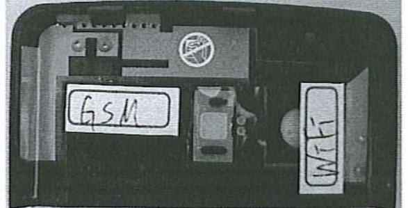
A grayscale photograph of the front cover of the X610 handset. The cover is dark with a vertical slot antenna on the left labeled "GSM" and a circular antenna on the right labeled "WiFi". |
