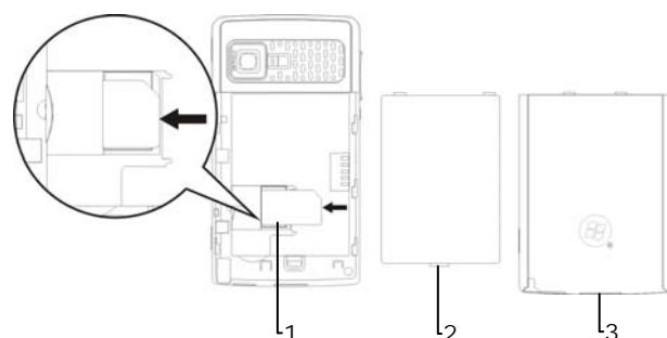
■ Installing the Battery
