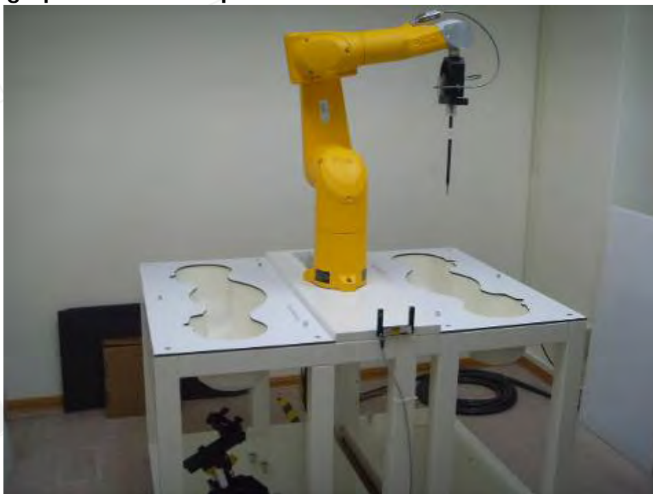
Fig.1 Photograph of the SAR measurement System
