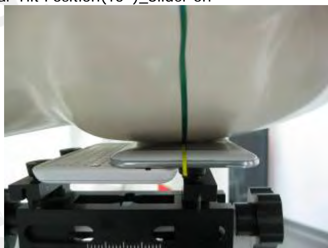
Fig.9 Left Head Section / Cheek-Touch Position_ Slider on
