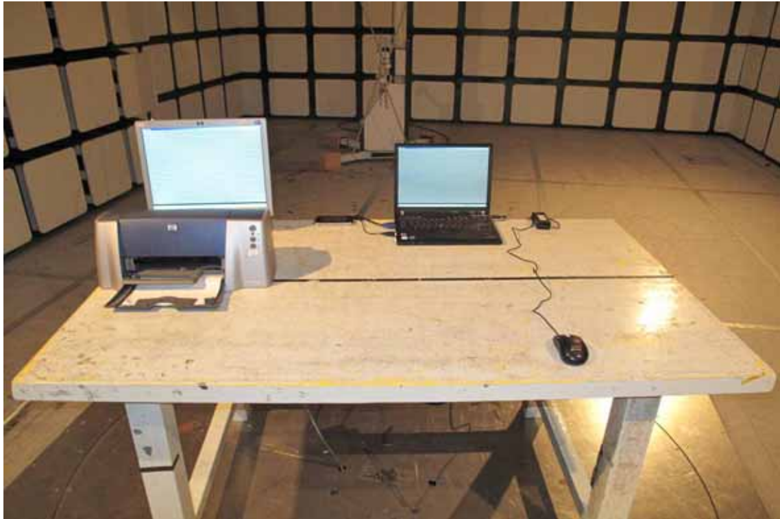
Radiated Emission Test Setup Photo (config 4)
