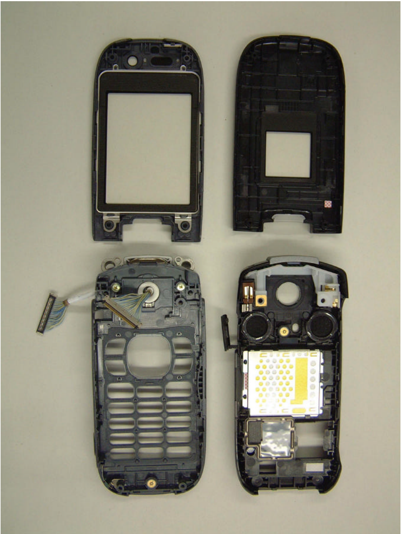
Upper Case and Lower Case (Inside View)
