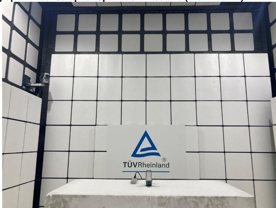
Photograph 2: Test Setup for Spurious Emissions (Front View 2)
