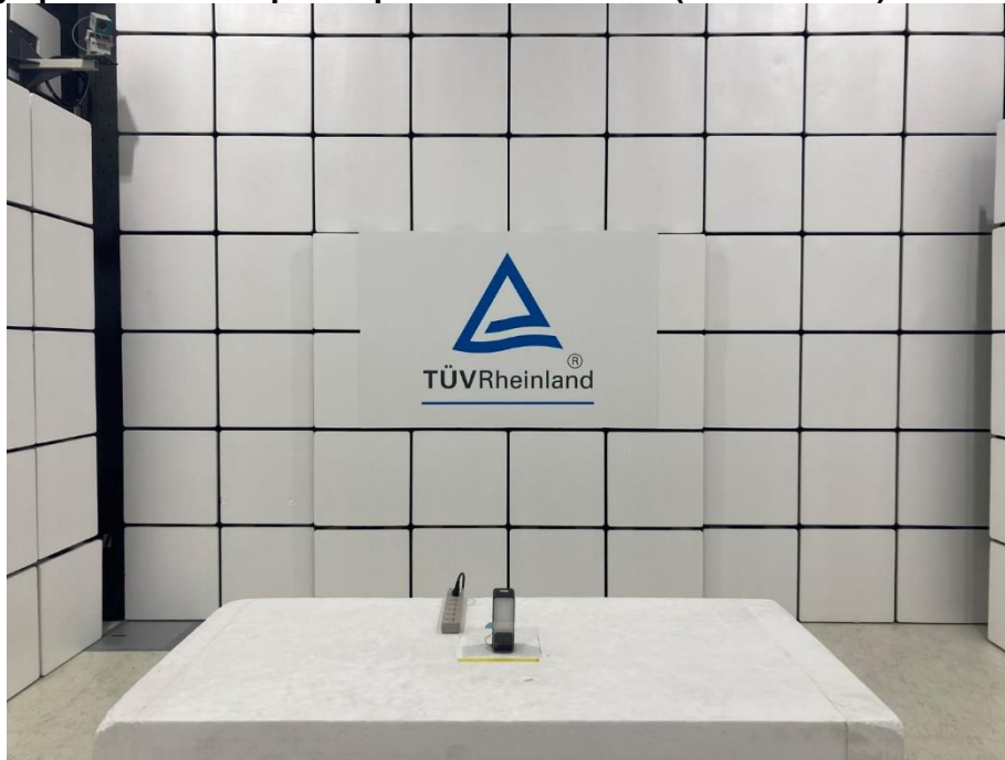
Photograph 2: Test Setup for Spurious Emissions (Front View 2)
