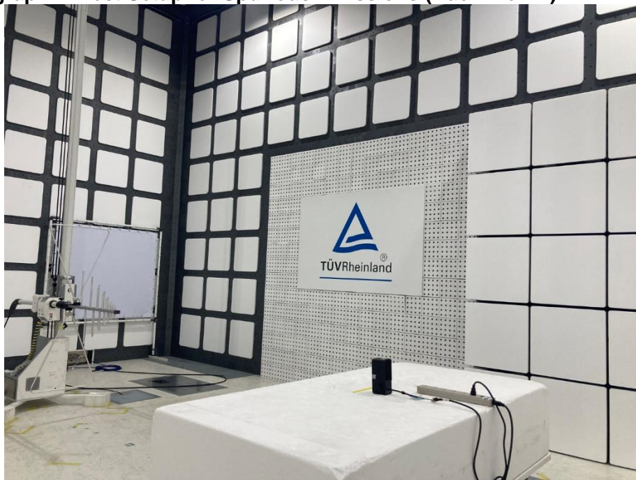
Photograph 4: Test Setup for Spurious Emissions (Back View 2)
