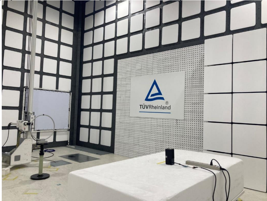
Photograph 4: Test Setup for Spurious Emissions (Back View 2)
