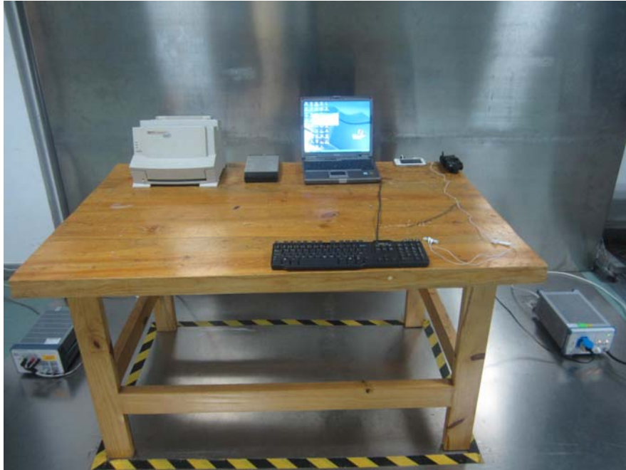
Conducted Emissions – Side View
