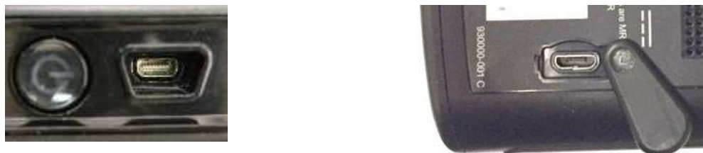
Figure 4. Argus 2s VPU – Detail: Cable ports Left: Connector for cable to OR Coil; Right: Connector for cable to computer (for programming, etc.)
