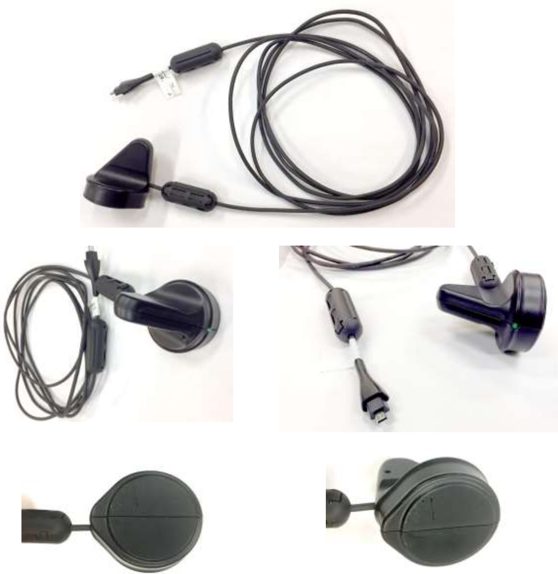
Figure 2. Argus 2s OR Coil (Transmitter) – various views Note: OR Coil Label, placed on the front surface of the coil, has been removed.
