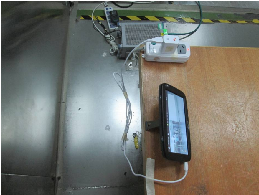
Conduction Emissions - Side View
